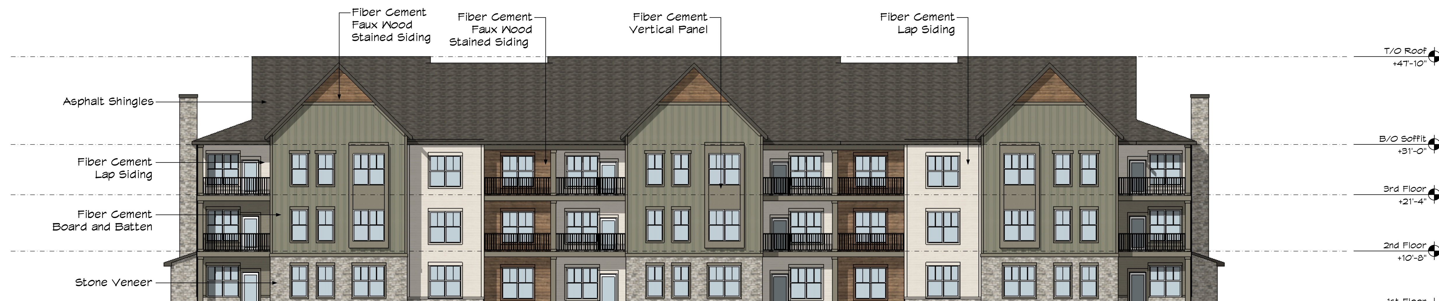
BACK ELEVATION - BUILDING TYPE A
