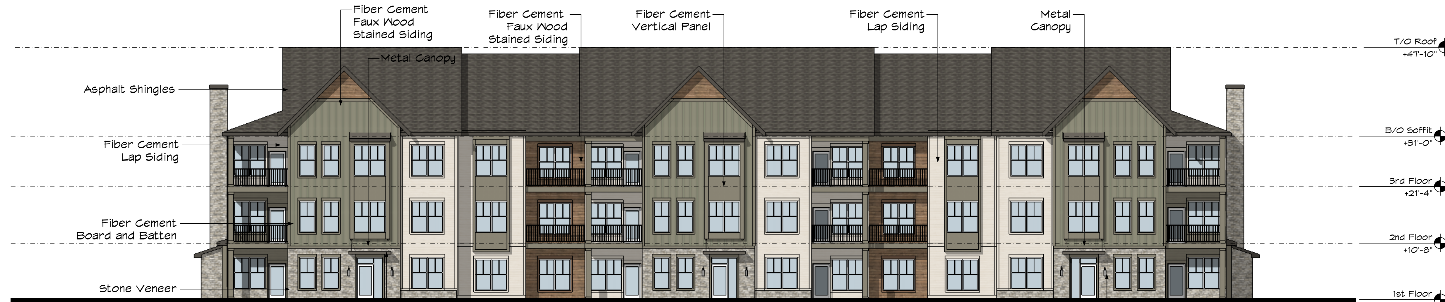
FRONT ELEVATION - BUILDING TYPE A
