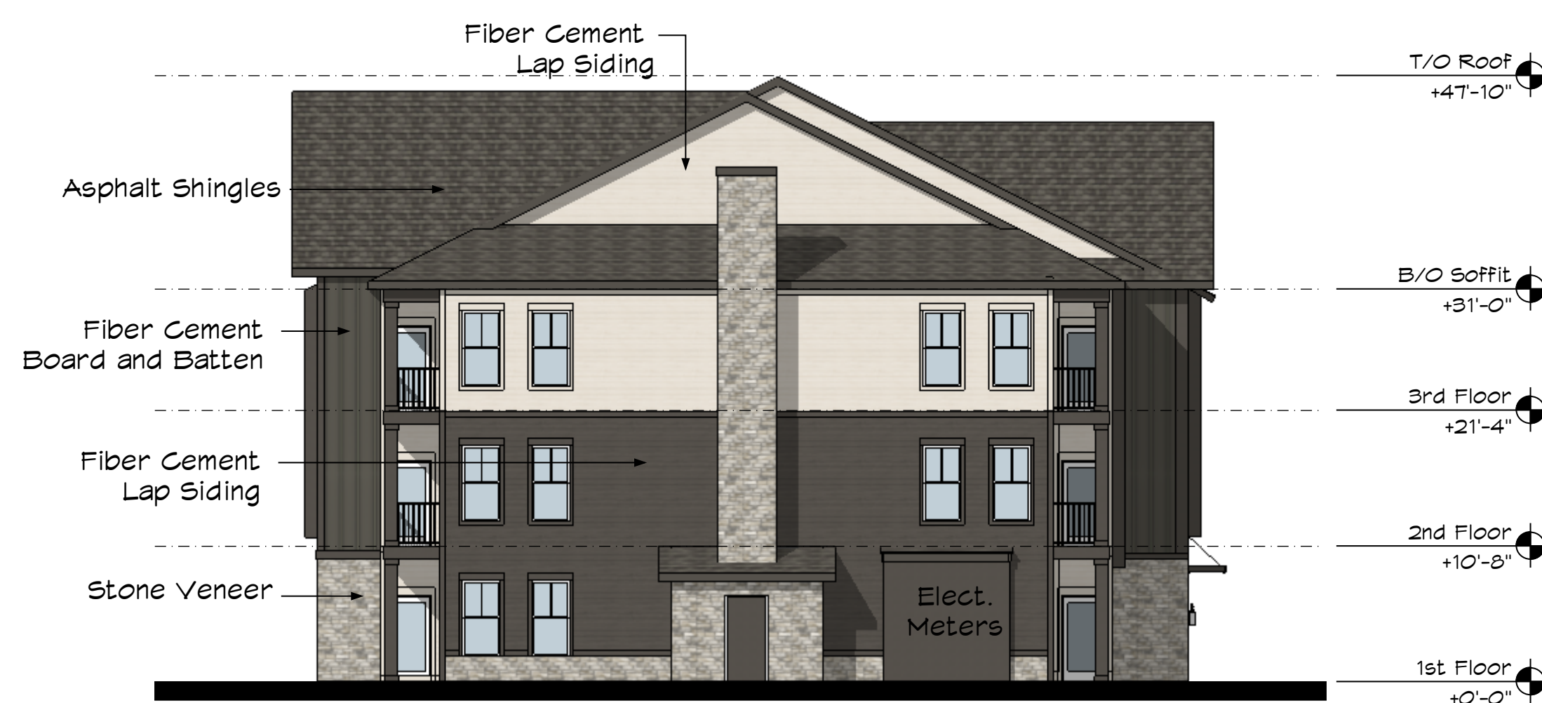
SIDE ELEVATION - BUILDING TYPE D
