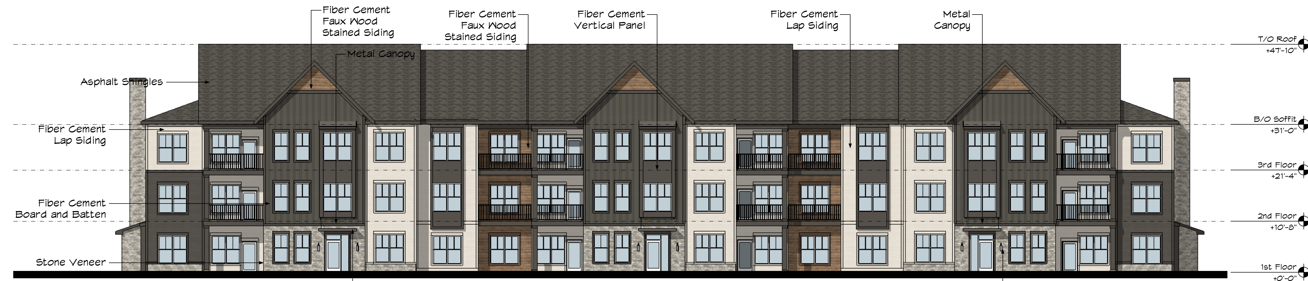
FRONT ELEVATION - BUILDING TYPE C
