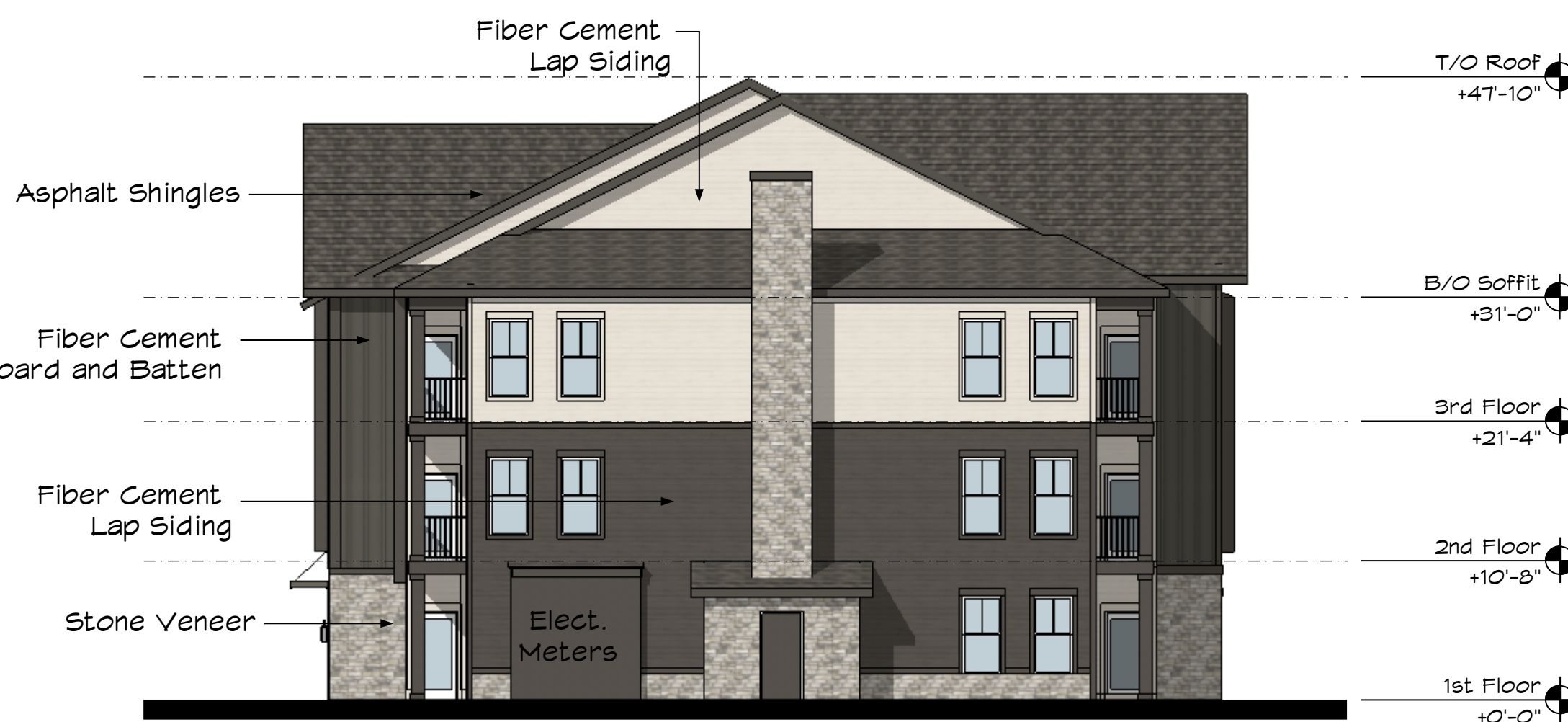
SIDE ELEVATION - BUILDING TYPE D
