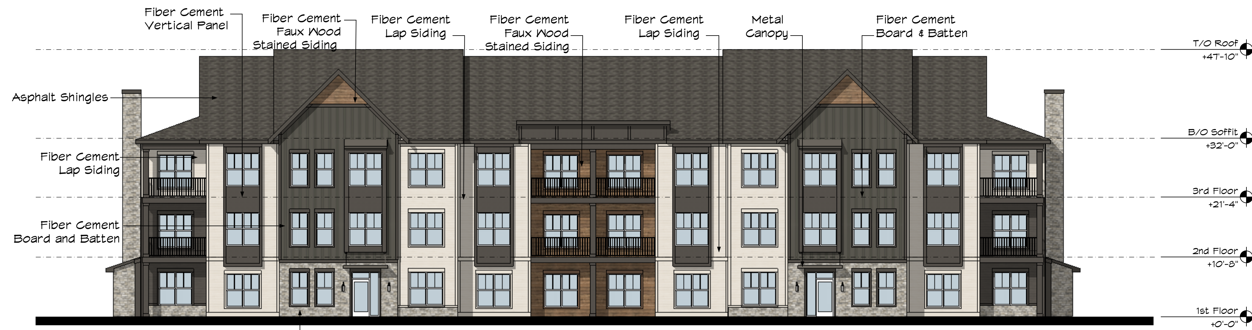
FRONT ELEVATION - BUILDING TYPE D
