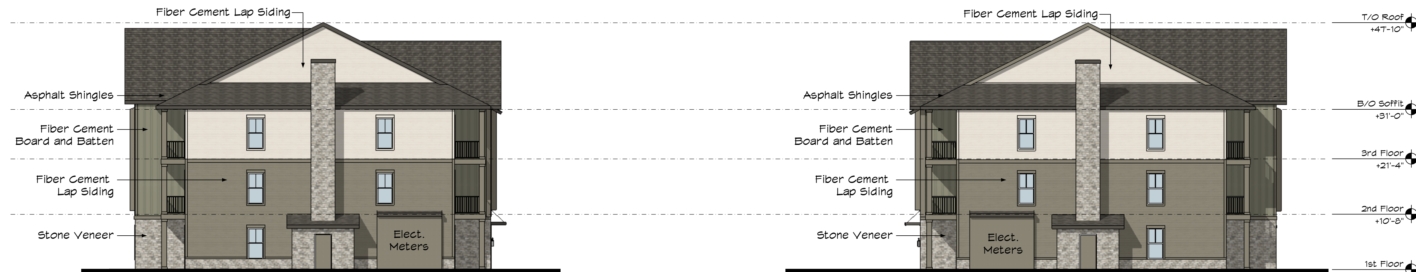
SIDE ELEVATION - BUILDING TYPE A
