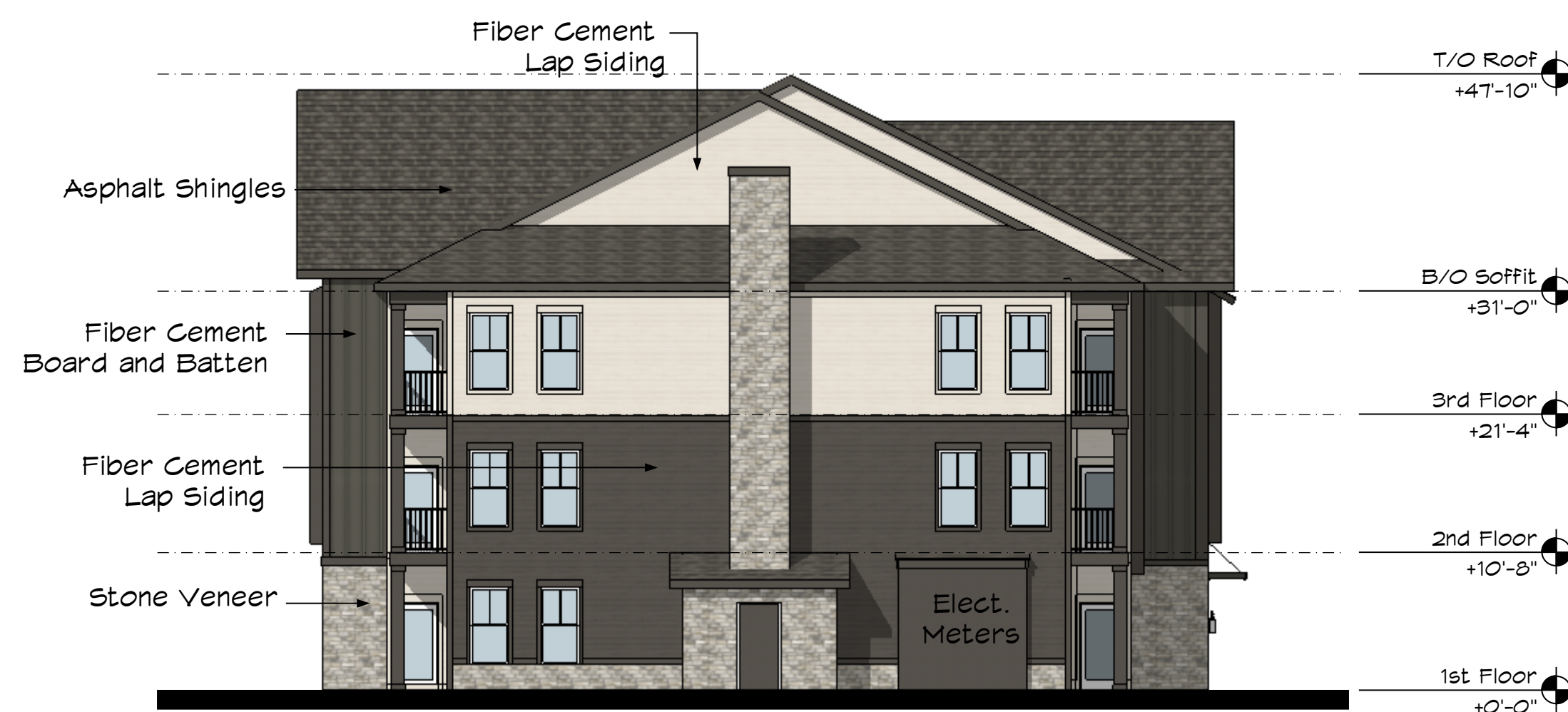
SIDE ELEVATION - BUILDING TYPE D
