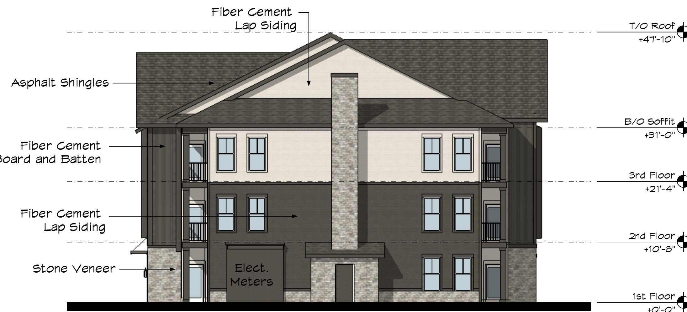
SIDE ELEVATION - BUILDING TYPE D
