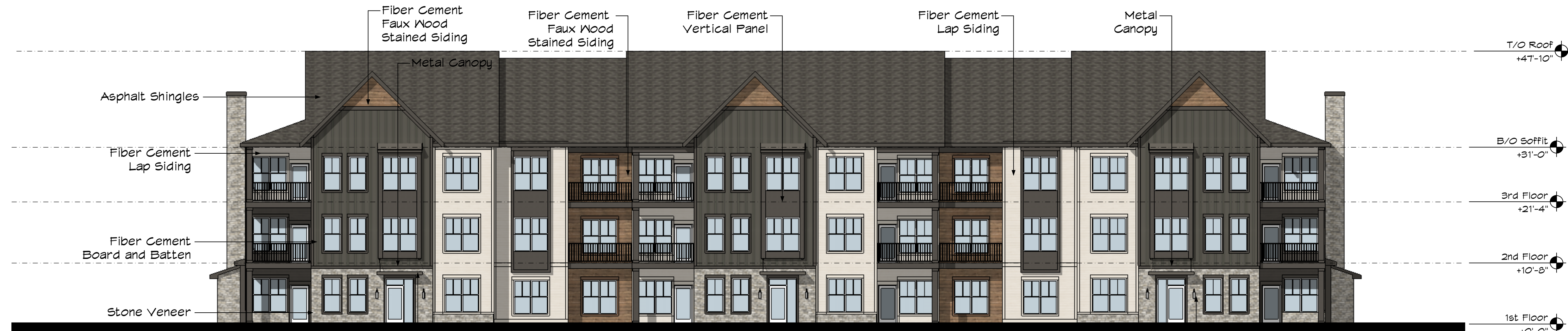
FRONT ELEVATION - BUILDING TYPE A
