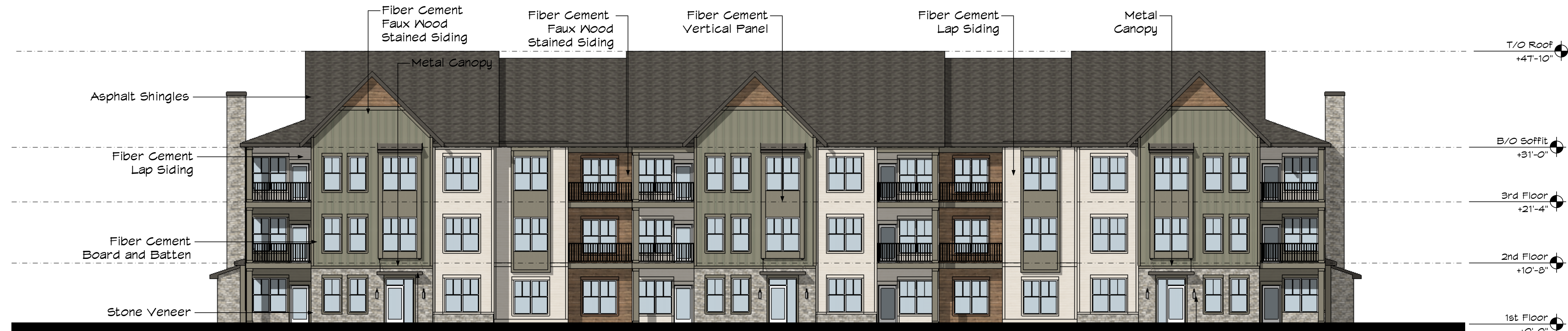
FRONT ELEVATION - BUILDING TYPE A
