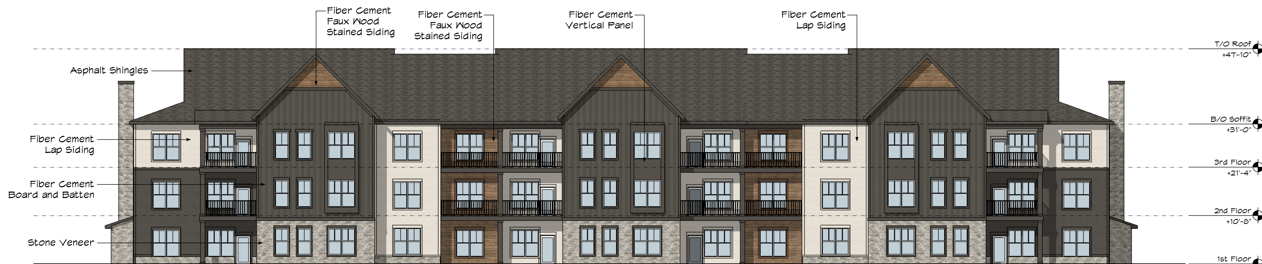
BACK ELEVATION - BUILDING TYPE C
