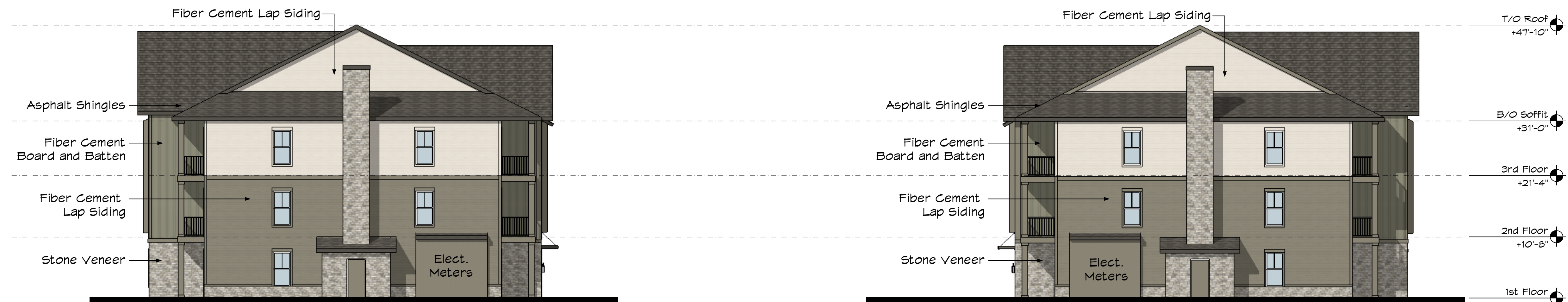
SIDE ELEVATION - BUILDING TYPE A
