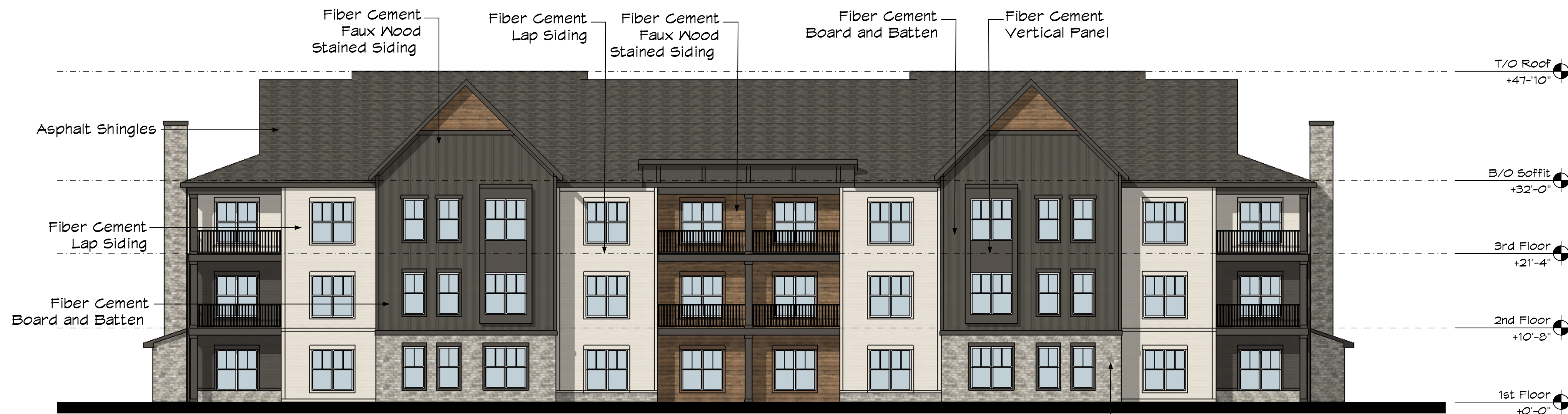
BACK ELEVATION - BUILDING TYPE D
