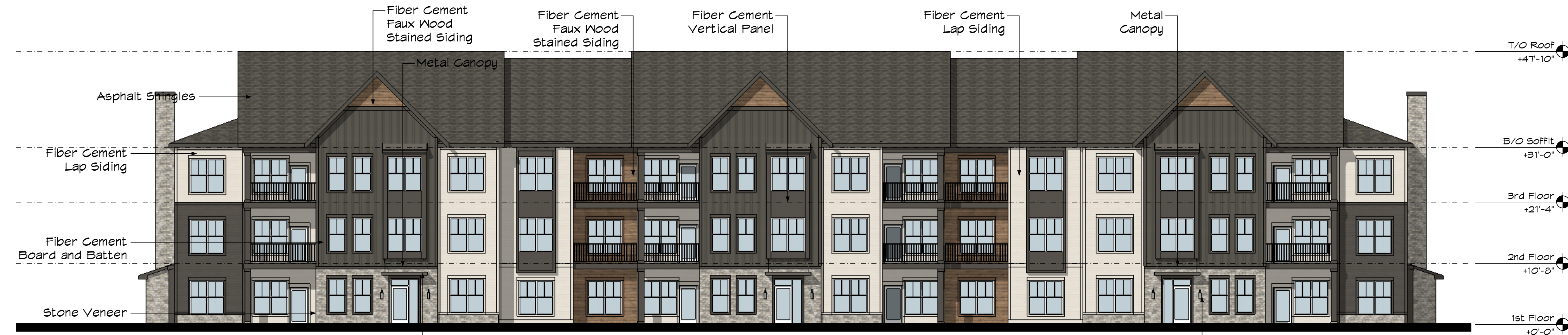
FRONT ELEVATION - BUILDING TYPE C
