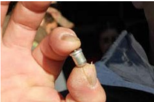
Mercury Switch from Vehicle Convenience Light
