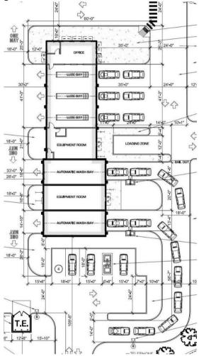
The illustration is the layout of the facility as proposed in our Development Permit. There is ample stacking. And staging areas to allow customers access to the various service offered. Also, we have two ingress and egress points to facilitate the operational needs and to reduce traffic to both Taco Bell and Walgreens.
