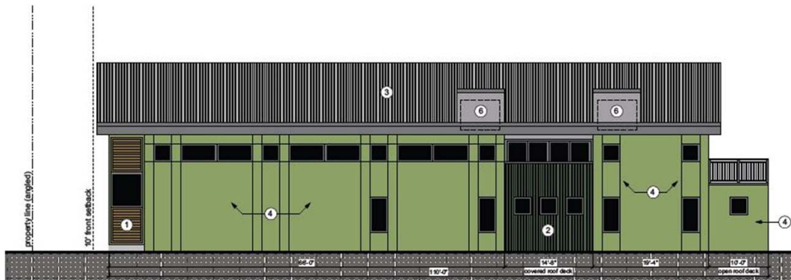
2 South Exterior Elevation 1/8" = 1'-0"
