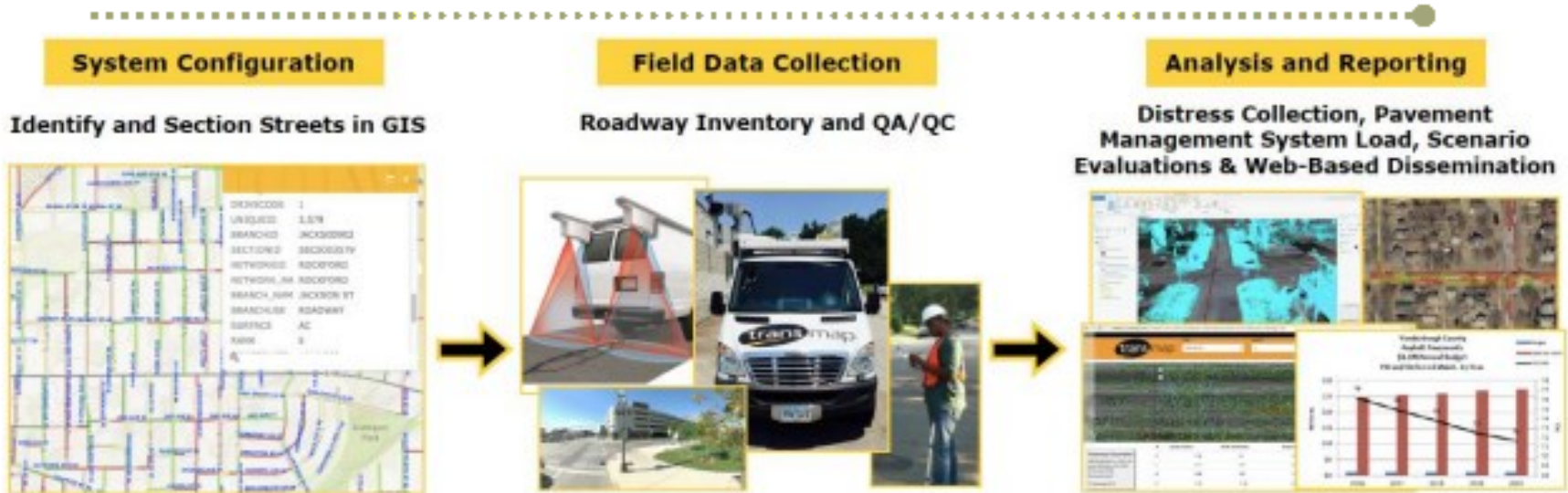
Figure 1-2 - The Pavement Management Process
