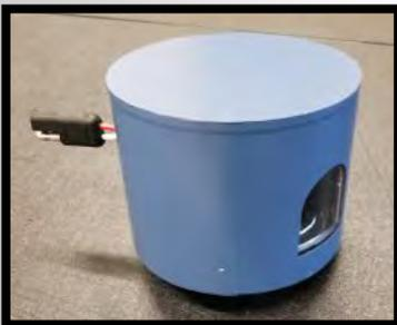
Sandoval Custom Creations Inc. produces a 12v Power-tap Photo-Sensor. The Power-tap Photo-Sensor can be utilized to power an enclosure on a light pole. The Power-tap Photo-Sensor supplies 12v-15w with a total of 1.3 amps. The Photo-Sensor still functions like a normal photo-sensor. This accessory from SCCI is a easy way to supply power to an enclosure.
