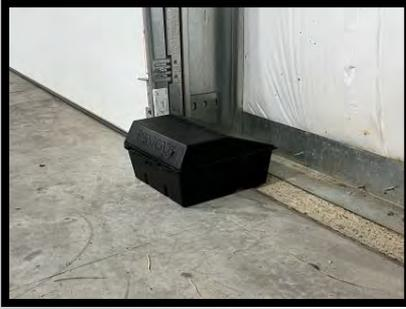
The Rat Trap-Cam is a battery powered concealment that uses a 1080p pin-hole camera and a cellular modem. This quick deployable system can blend into a warehouse setting or in a industrial area. With the Rat Trap-Cam you can remotely access the live video through a cellular modem. The battery will provide 2.5 days of run time with a cellular modem and camera. The best part of the Rat Trap-Cam is no one will want to touch it once deployed!
