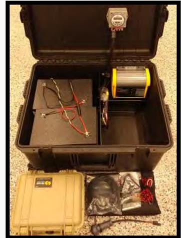
***WARNING: AGM batteries must be used in this system. Using standard batteries can result in an explosion.***
