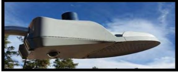
The Leotek LED Street Light is another model of LED street light. This system features the Axis M5065 or Canon VB-S30D PTZ, micro dome, full HD network camera that is powered by POE and contains a Sierra Wireless LX40 modem or similar size modem. All internal components are mounted to SCCI's specifically designed, 3D printed, carbon fiber infused PLA bracket.
