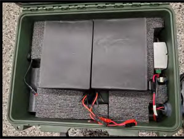
Our Dual LiFePO4 Battery Pack is contained in a Pelican Storm case. The HPX® high performance resin gives a solid base for electronic/structural installation and durability. The Dual LiFePO4 Battery Pack is designed to be weather resistant and able to
