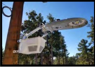
This enclosure replicates a Metropolitan communications box. The Metricom-Cam features a swivel bracket and adjustable hanging arms. This unit has three windows to maximize the field of view. The enclosure has power venting to keep electronic components cool. This system
