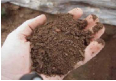
Compost blankets can be used in areas not subject to concentrated flows and shall be applied with a pneumatic blower or by hand.
