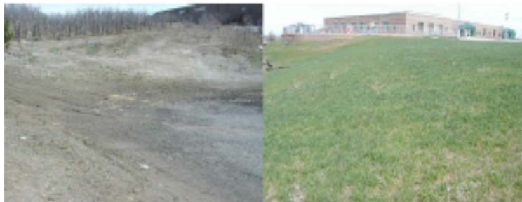
The area on the left was hydraulic seeded at the same time as the area on the right (across the street) was drilled. Due to poor performances like this example, Hydraulic seeding/mulching is not allowed as a seeding method.
