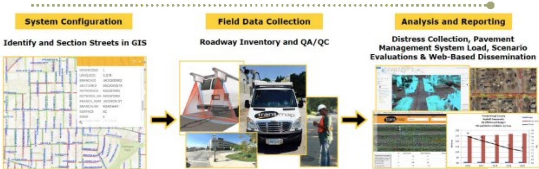
Figure 1-2 - The Pavement Management Process
