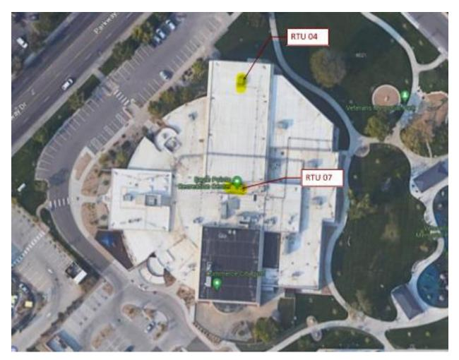
There is no screening wall for either unit, however a block wall is in close proximity to RTU #7. Staging for crane access must be approved by the Owner prior to commencement of work.
