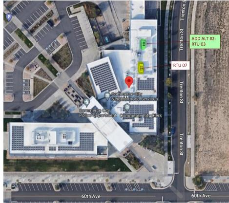
The existing model for AHU #7 is a 50 Ton Aaon (RN-060-3-0BA02-EJL) conditioned water, heat pump system. The existing rooftop unit is supported by a mechanical curb platform and is surrounded by a screen wall system. The existing curb footprint shall be maintained and re-utilized. If the curb must be
