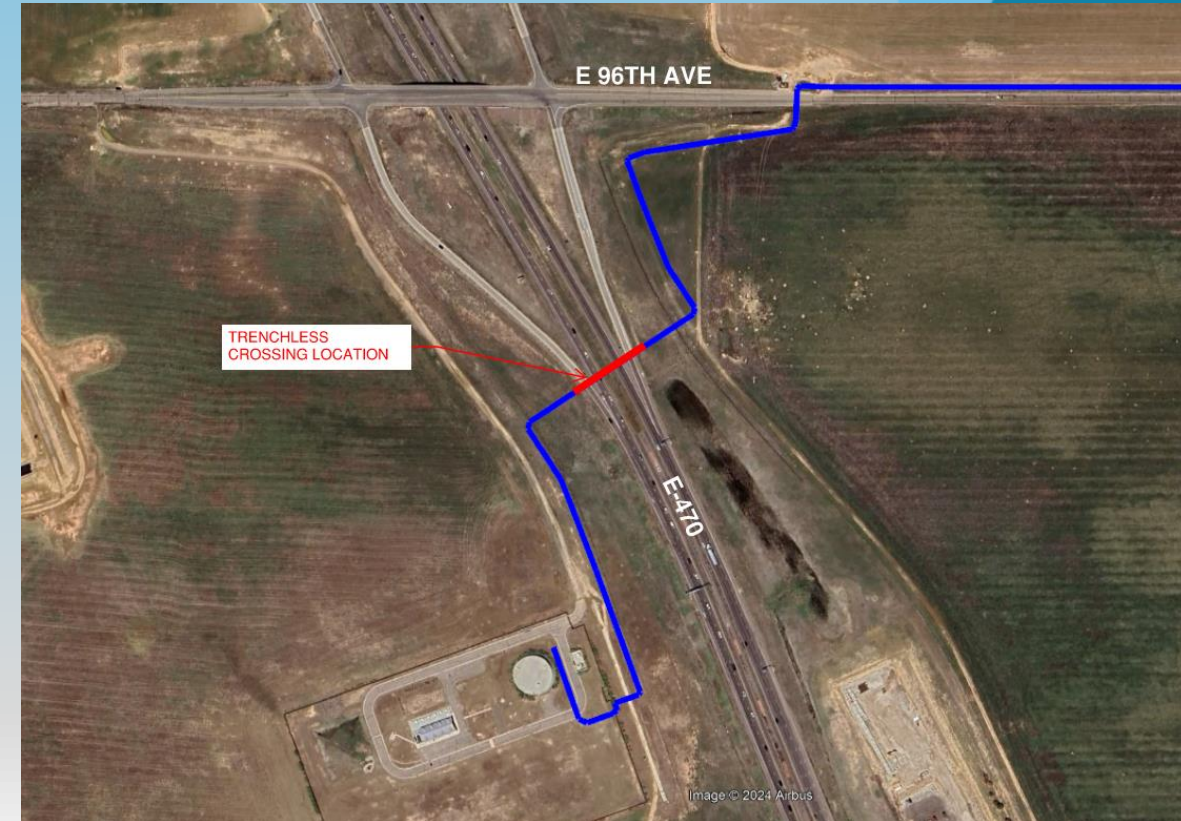
Trenchless Installation of 48" Steel Casing
