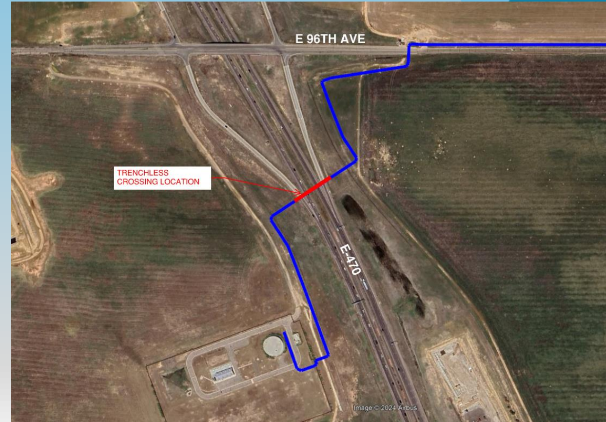
Trenchless Installation of 48" Steel Casing
